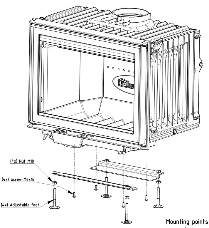
Install the mountingplate with the bolts on the bottom plate (see figure)
